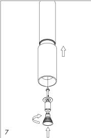
Lift the brass and wood part. Insert the GU10 bulb.
