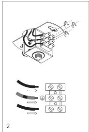
Connect the cable to the terminal block.
