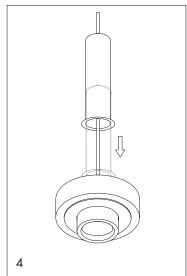
Insert the cable into the copper tube all thought until the base part of the tube make contact with the top part of the stone.
