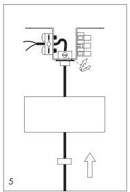
Fix the lamp cable with the fixing plastic screw on the ceiling box. Take care to screw gently but firmly.
