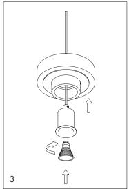
Attach the Gu10 LED bulb into the socket and then insert the cable into the stone.
