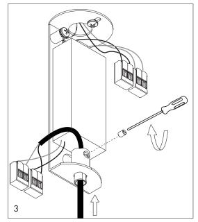
Fix the lamp cable in the right height with the fixing bracker on the side to doble secure.
