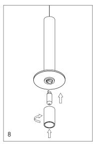
Insert the G9 bulb and screw in the metal tube.
