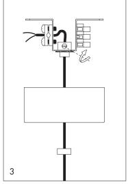
Fix the lamp cable with the fixing screw on the ceiling box. Take care to screw the screw gently but firmly
