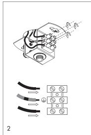
Connect the cable to the terminal block.
